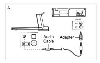
B. Plug one end of the audio cable into the jack on the front of the treadmill near the power cord. Plug the other end of the cable into the included adapter. Plug the adapter into an RCA Y-adapter (available at electronics stores). Next, remove the wire that is currently plugged into the AUDIO OUT jack on your VCR and plug the wire into the unused side of the RCA Y-adapter. Plug the RCA Y-adapter into the AUDIO OUT jack on your VCR.
